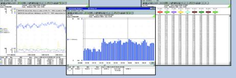
**Event data** read out from one or several MAVALOGs are listed in the order in which they occurred and can be printed out in report form. In the event of voltage dips, interruptions or swells, these are displayed in a Y-T diagram and can be analyzed with the cursors.
